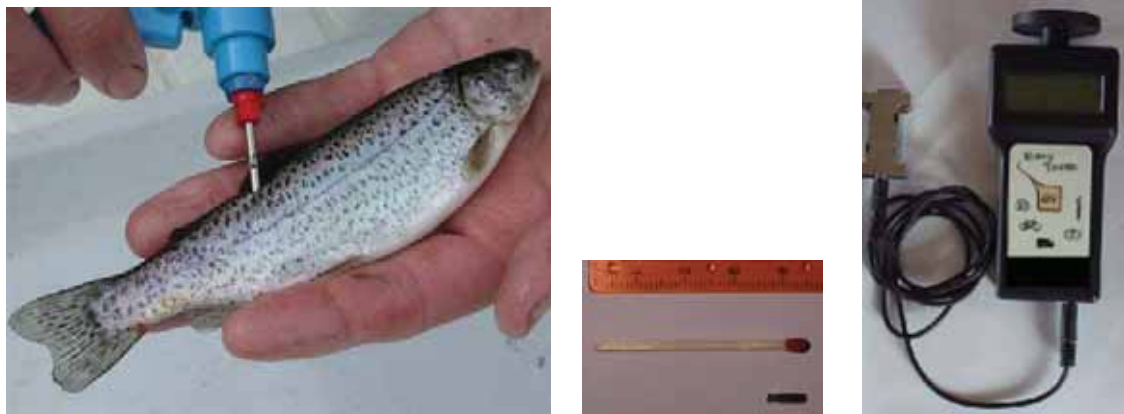
Figure 3. Injection of a PIT tag in the fish (left); PIT tag in the lower right corner (middle); and a scanner (right). Photo: Torben Nielsen and Alfred Jokumsen.
