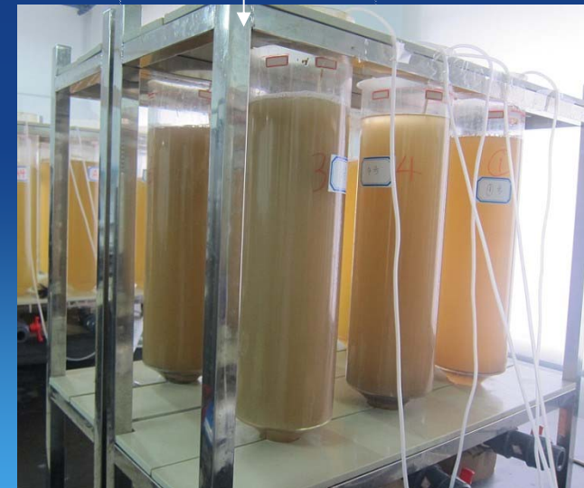
Lab-scale external biofloc reactors
