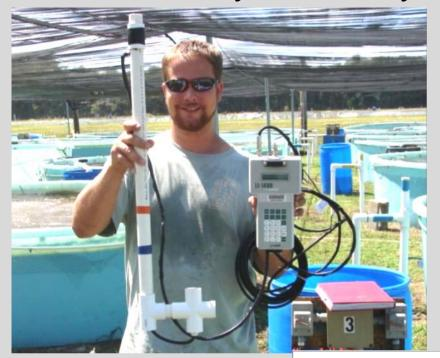
Hand held light meter; one sensor above the water surface, the other 20cm below
